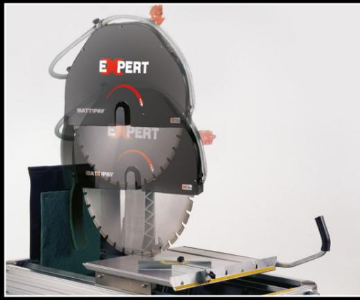
The cutting head is tilting and can be locked at the intended height.
